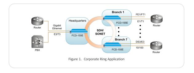
SDH/SONET media can transport basic Ethernet packets of up to 1536 bytes enabling connection to MPLS networks.
