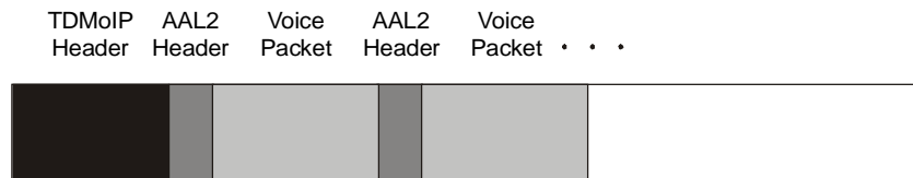
Figure 1-10. TDMoIP Frame Structure
