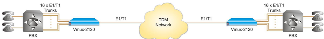
Figure 6. Vmux-2120 Transporting up to 496/384 Voice Channels over a Single TDM Link
