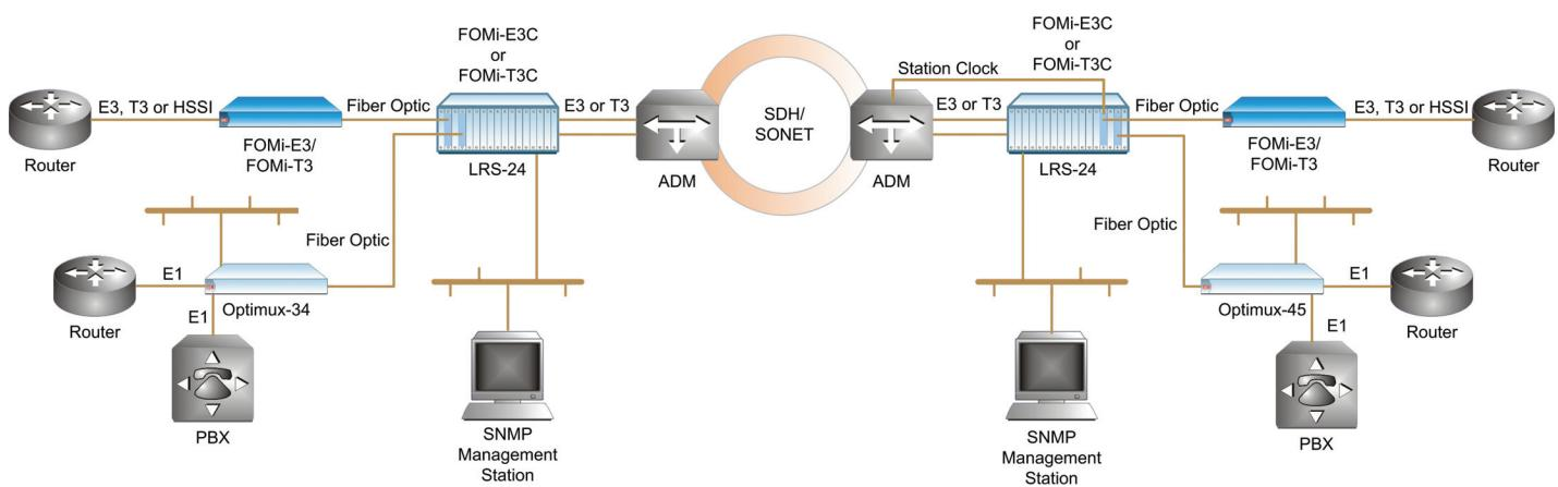
Figure 1. FOMi-E3 or FOMi-T3 Working Opposite RAD's Optimux Multiplexers
