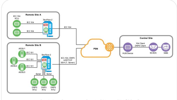
Figure 1. Connecting Legacy RTUs, Using Protocol Gateway and Stateful Firewall
