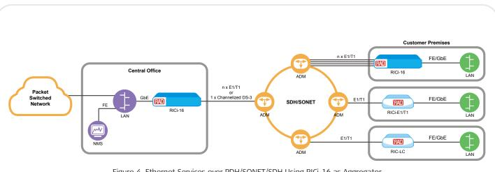
Figure 4. Ethernet Services over PDH/SONET/SDH Using RICi-16 as Aggregator
